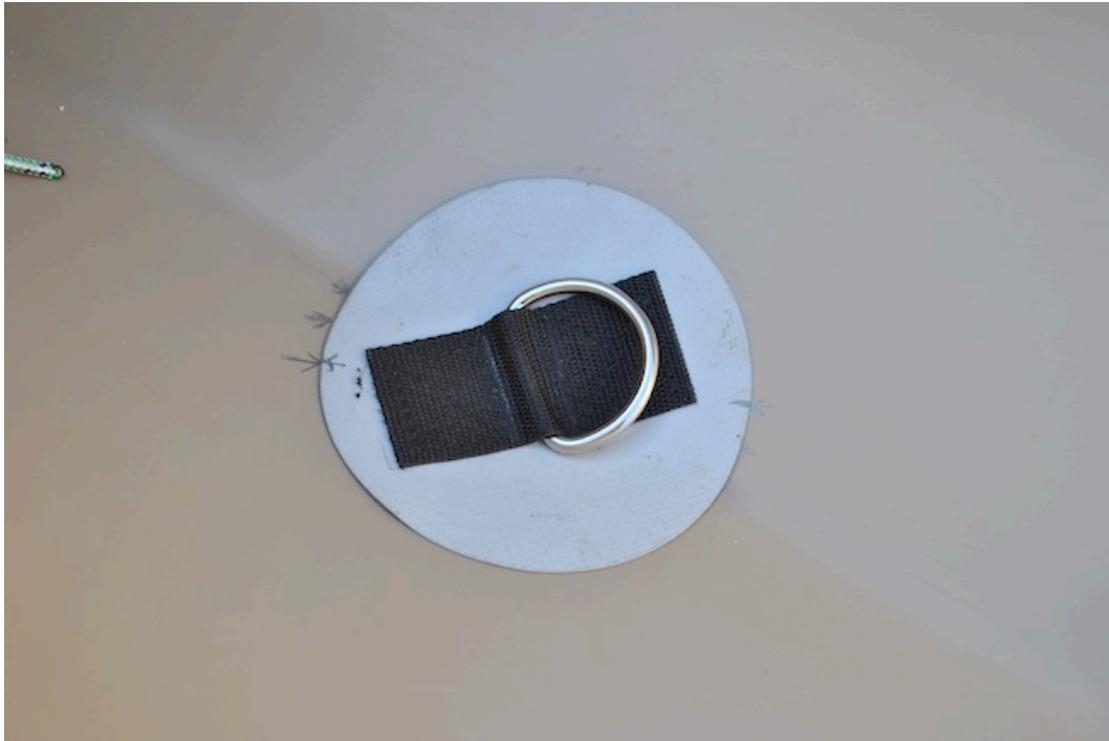
I use my inflated air bags to work out exactly where I want the rings and draw round them. I have used large 2" rings for this job. Note the angle I have had to set the rings at in order to accommodate the shallow 'V' of the hull.
