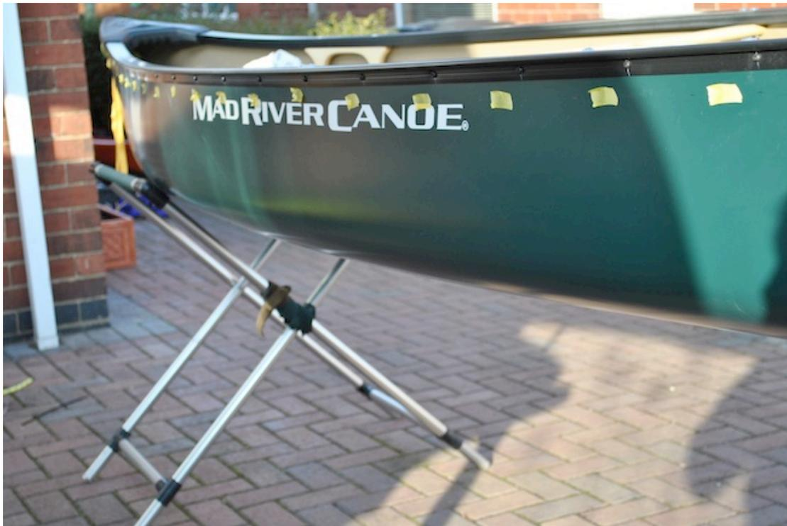
As I intend to lace the entire length of the boat I start at the centre of the boat marking holes either side of the ends of the Yoke. I then continue this process down both sides of the boat and to each end marking where the cord loops will be on the outside with yellow tape. Remember to make sure that the end of the cord should end up inside the boat at the last hole.
