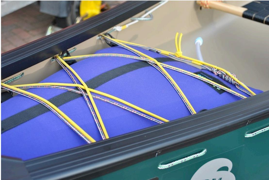
I have also added some shock cord over the bags for tucking a spare paddle and swim lines etc under. Note I don't recommend using only shock cord to secure your airbags, as this will allow too much movement in the bags, possibly resulting in the air bag being popped out when swamped.
