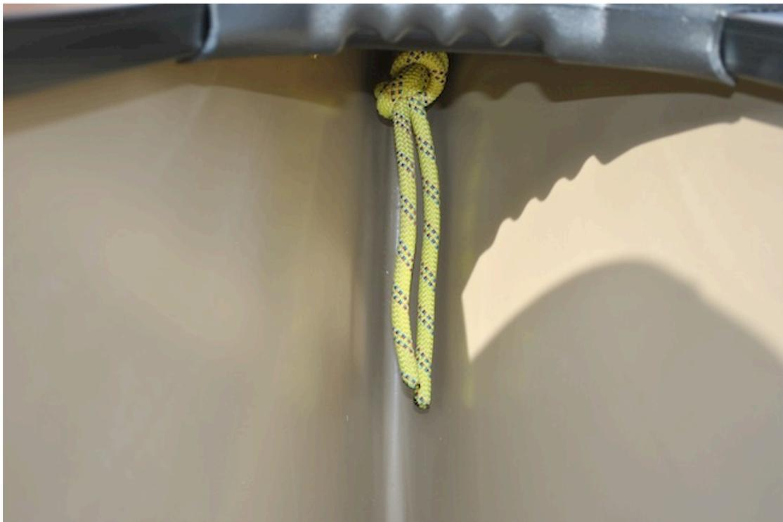
At this point I make sure that the loop on the outside is snug to the hull before tying a overhand knot on the bight close up to the inside.
