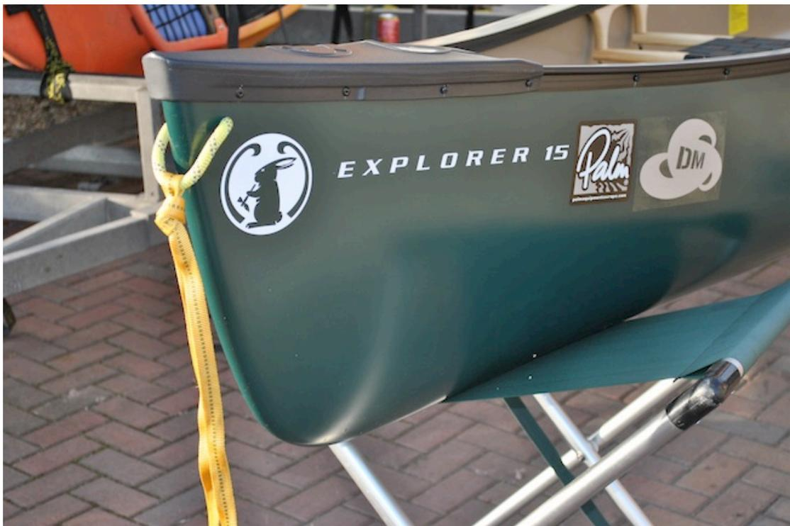
The finished article above with the swim tail fitted. Note the small size of the grab loop. If you are going to attach painters remember that they go through this loop, and can be either permanently attached or removable for transporting. As for length then it is again very much down to personal choice and how/where you will be using your boat. I would suggest as a minimum, a boats length of floating rope. If you choose longer then consider how you will
