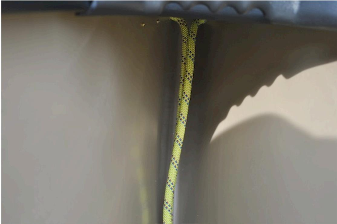
Once drilled and cleaned out, thread your rope through so that both ends of the rope end up inside of the bow and below the deck plate.
