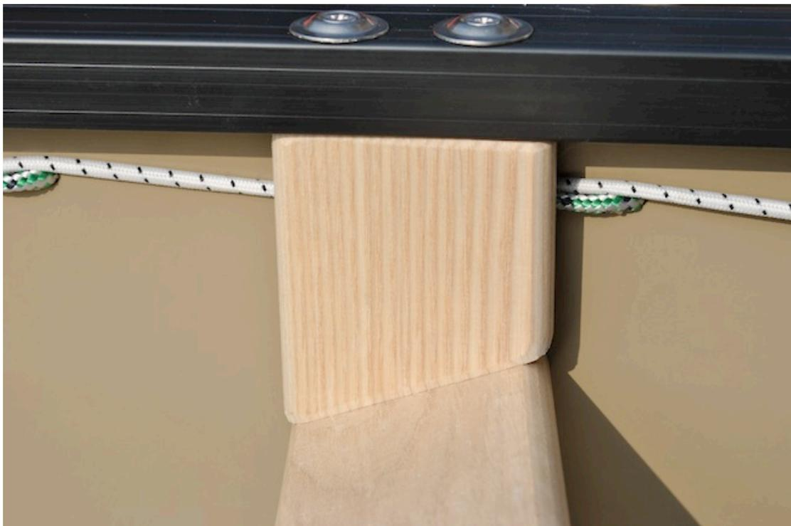
Before finally assembling your thwart it is a good idea to give all the wooden parts, especially where you have trimmed them a good couple of coats of Boiled Linseed oil. For this I use a 50/50 mix of Boiled Linseed and White Spirit. Leave each coat to soak in and then buff vigorously with a cloth before completely dry in order to remove any excess. The heat generated by the rubbing will also help the oil soak in.
