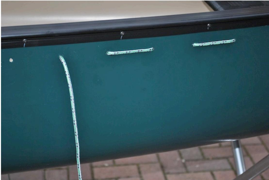
I used a 5mm drill bit so that the cord (also 5mm) is a snug fit. With the holes drilled I start at one end, and secure with a knot on the inside then begin to lace down the sides of the boat using 5mm cord. I personally would not use anything less than 5mm cord for the lacing as it could slice through the plastic like a cheese wire.
